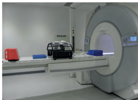
FIGURE 2. (left) In-house manufactured coils support for pelvis imaging; (right) the couch securing mechanism with adjustable size
