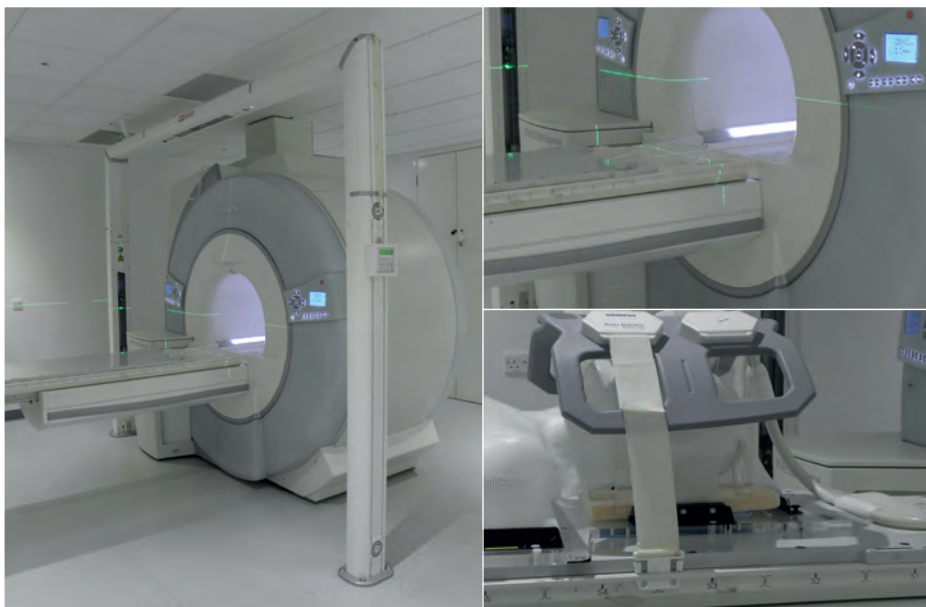
FIGURE 1. (left) Medibord RT flat couch top; (top right) access to head coil fixtures; (bottom right) retaining access to coil-securing fixtures and utilising these fixtures for securing the couch top in position
