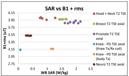
Figure 1: Measured whole body SAR and B1+rms at different table positions.
