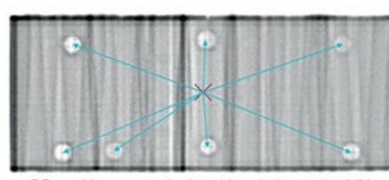
BB positions are calculated in relation to the MV center. Remember the MV center is known from the MVGeometry file.
