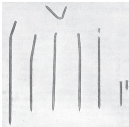
② Bent and broken radium needles. Hopwood & Smallwood *BJR* (1929).
