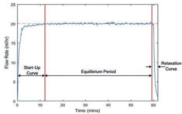
it was observed that the measured flow rate was below the set flow rate during the entire infusion period. The start-up times are particularly relevant when infusing drugs such as Dopamine, which metabolises quickly. It is vital that drugs such as these reach the patient as soon as possible and delays in delivering the drug could have harmful effects on the patient.
