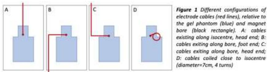
**Results** The maximum recorded temperature rise measured at the electrode needles was 3.2°C after 15 mins (Fig 2A); this was with the electrode cables running along the isocentre (Fig 1A). On average, the temperature rise was slightly higher when the cables exited the scanner along the isocentre (mean  $dT = 2.5$  °C), compared to when the cables were adjacent to the scanner bore (mean  $dT = 2.0$  °C; Fig 2B).
