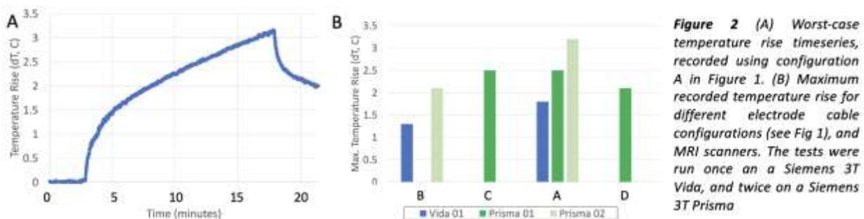
**Figure 2** (A) Worst-case temperature rise timeseries, recorded using configuration A in Figure 1. (B) Maximum recorded temperature rise for different electrode cable configurations (see Fig 1), and MRI scanners. The tests were run once on a Siemens 3T Vida, and twice on a Siemens 3T Prisma
