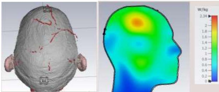
Figure 1 (a) Cranial plates placed on skull of Duke model, (b) SAR distribution for 8W input power.
