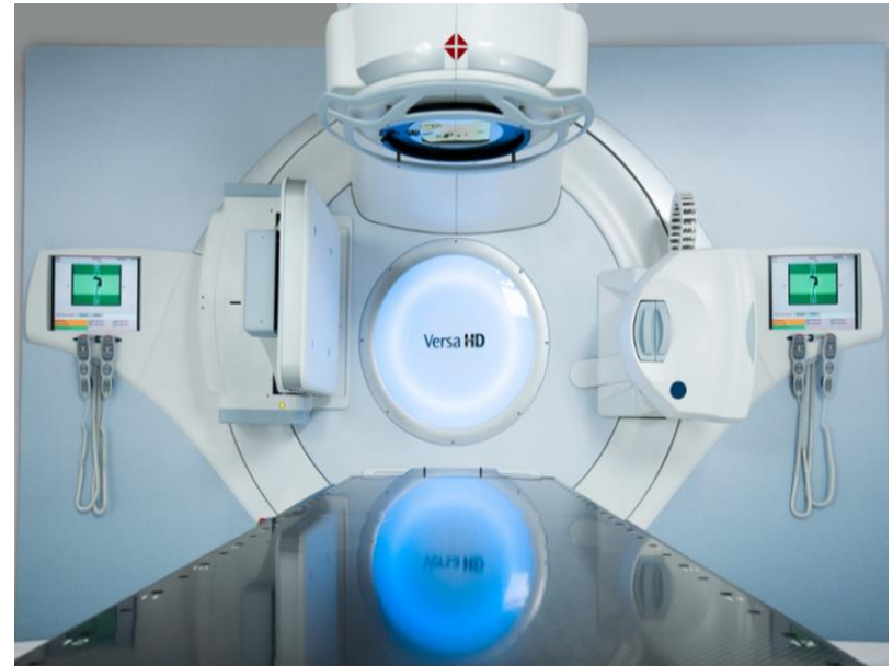
Elekta Versa HD linac 6 & 10MV, max 22Gy/min Max 40x40cm field
