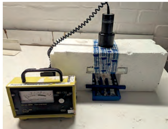
Figure 7 Monitor set-up for the radioassay calibration jig
