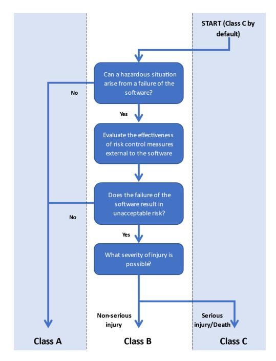
Figure A1: The process for determining the IEC 62304 software safety class
