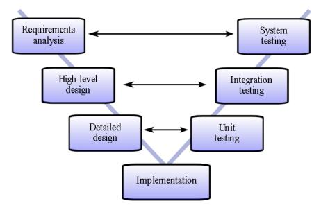
Figure A2: The V-model, which is similar to the Waterfall model, but has a strong emphasis on testing against each level of the device design (Bruyninckx 2008).
