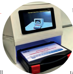
Figure 6 Working Prototype of the barcode scanner
